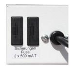
The two fuses for the shaker are located in a drawer below the device plug. To check and replace these fuses, the drawer can be pulled out after actuating the retaining levers on both sides. The fuses may only be replaced with fuses of the same construction. Information about the type of fuse used can be found on the nameplate next to the device socket and in the circuit diagram.
